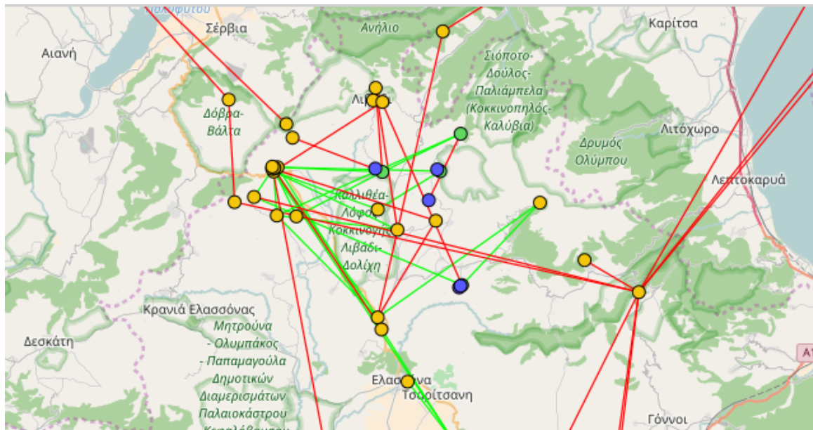
Figure 6.2: The green links correspond to the backbone network of Sarantaporo.gr CN interconnecting 14 villages in the Sarantaporo valey and including a long-distance link to the Internet gateway in Larissa (bottom)
